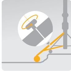
Levelling leg available in all the stands for ease of use on all different floor types. A fundamental feature for outdoor applications.
