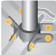
All the components are assembled using bolts (no rivets) for extra rigidity and easy maintenance if required.
