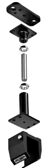
RIDIU Adjustable spacer between ceiling and RIGUE or RIGOE bracket. With 2 nuts (not including bracket or threaded rod). Adjustable up to 3 cm. Weight: 610 g
